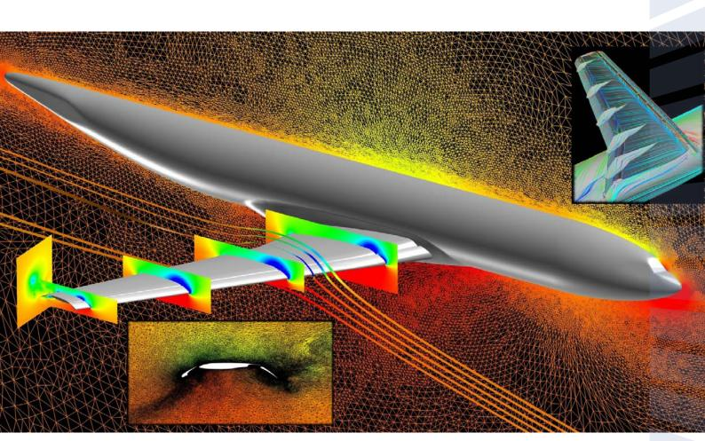
A computational fluid dynamics (CFD) visualization produced using a NASA supercomputer, showing a mesh adaptation used to simulate a transport aircraft NASA / Elizabeth Lee-Rausch, Michael Park http://www.nasa.gov/aero/aeronautical-simulation.html
