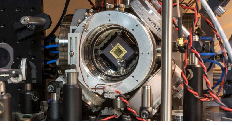
Ion trap on a microchip for quantum computing set inside a vacuum system in the Oxford Physics Lab / *Stuart Bebb*
